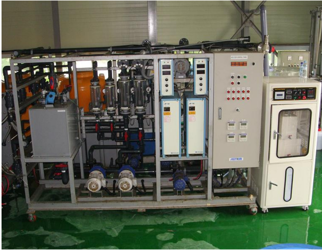
Fig. 3. Electro-dialysis desalination system for mineral control in deep seawater.
