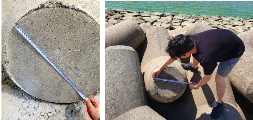
Fig. 5. Scene measuring D3 size of the wave dissipation block.
