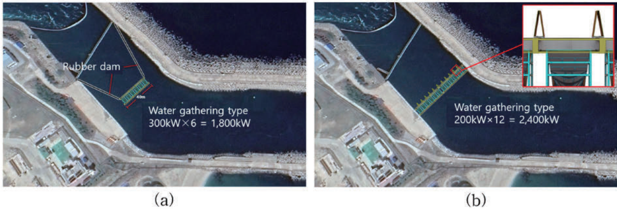
Fig. 8. Schematic diagram of the small hydropower generation in discharge channel (a: Case 1[1.8 MW], b: Case 2[2.4 MW]).
