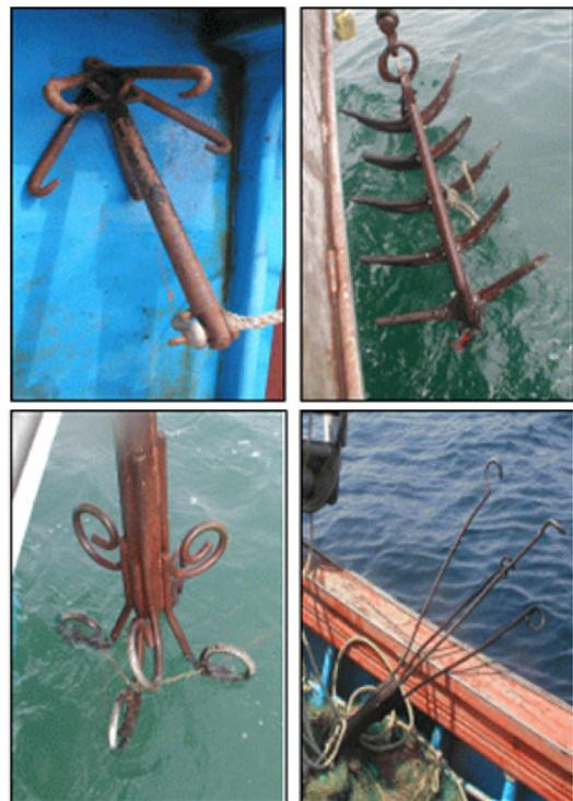
Fig. 2. The collecting gears used in this survey (from left to right, for mud, muddy sand, sand, and rock sea bed, respectively).
