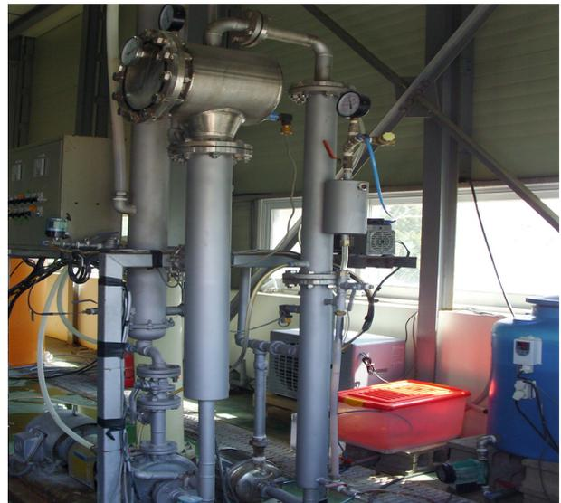
Fig. 2. Reduced pressure evaporation device.
