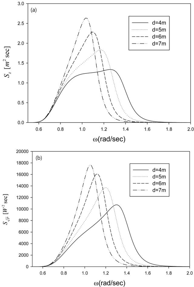
Fig. 9. (a) Heave motion spectrum and (b) square root power spectrum under the optimal condition ( $c_{PTO}=b_T$ ) as a function of draft and wave frequency for  $H_{1/3}=3.0$  m,  $T_p=6.67$  sec,  $a=2.0$  m,  $\kappa=0.053$ .
