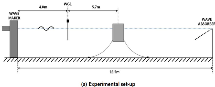
Fig. 3. Experimental set-up and circular cylinder buoy.
