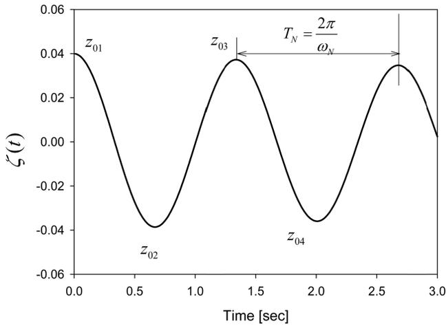
Fig. 2. Time series of heave free-decay test.
