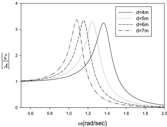
Fig. 5. Heave RAO of a buoy in case of disconnected generator ( $c_{PTO}=0$ ) as a function of draft and wave frequency for  $h=80$  m,  $a=2.0$  m,  $\kappa=0.053$ .
