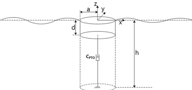
Fig. 1. Definition sketch of a WEC in waves.
