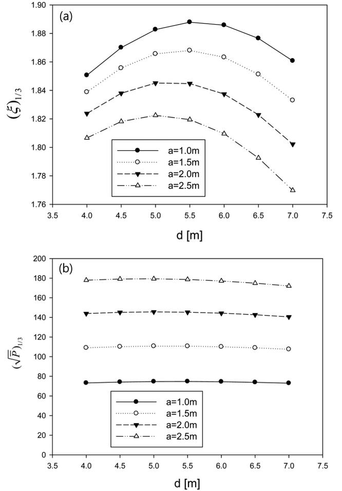
Fig. 10. (a) Significant heave amplitude and (b) significant amplitude of square root power under the optimal condition ( $c_{PTO}=b_T$ ) as a function of draft and radius of a buoy for  $H_{1/3}=3.0$  m,  $T_p=6.67$  sec.
