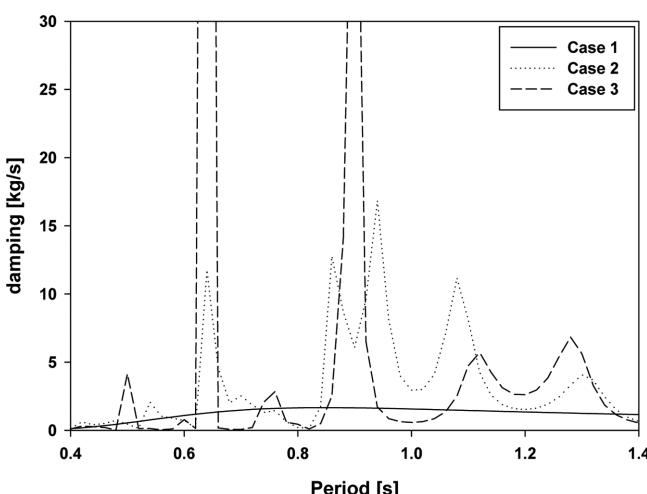
Fig. 6. Radiation damping coefficients.
