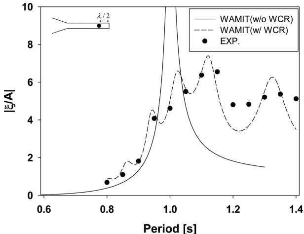
Fig. 9. Comparison of heave RAO between numerical solutions and experimental results with and without a water channel resonator for single Cyl-2 cylinder ( $b_{vis} = 2.2405 \text{ kg/s}$ ).
