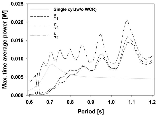
Fig. 14. Time average power with an optimum PTO damping coefficient.
