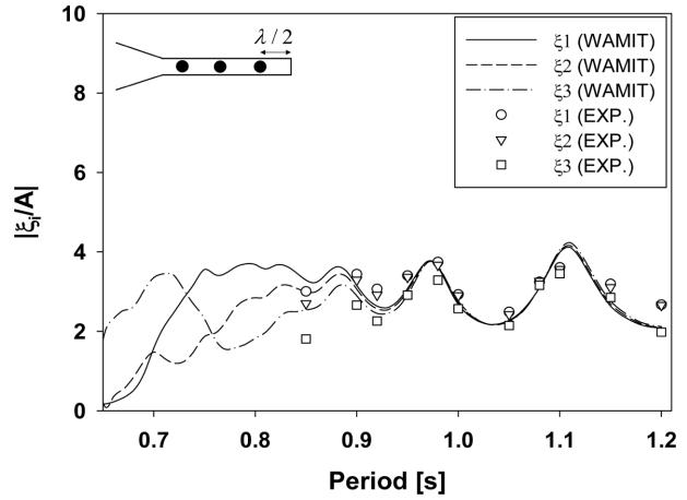
Fig. 10. Comparison of heave RAO between numerical solutions and experimental results for three Cyl-1 cylinders arrayed in a water channel resonator.
