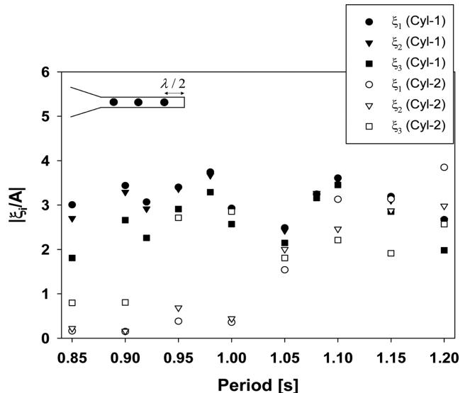
Fig. 11. Experimental results for heave RAO between three Cyl-1 and Cyl-2 arrayed in a water channel resonator.
