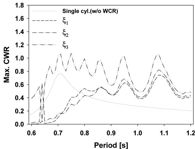
Fig. 15. Capture width ratio with an optimum PTO damping coefficient.
