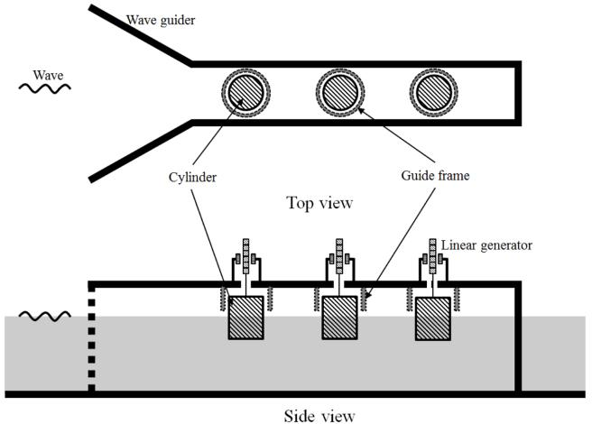
Fig. 1. Multiple wave energy converters in a water channel resonator.
