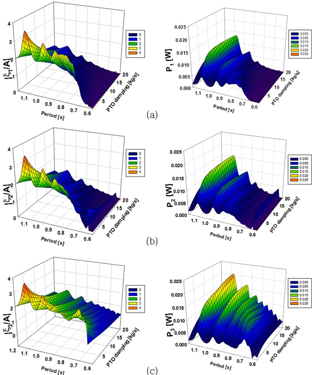
Fig. 12. Heave RAO(left) and time average power(right) as a function of periods and PTO damping coefficients at three Cyl-1 cylinders arrayed in a water channel resonator.
