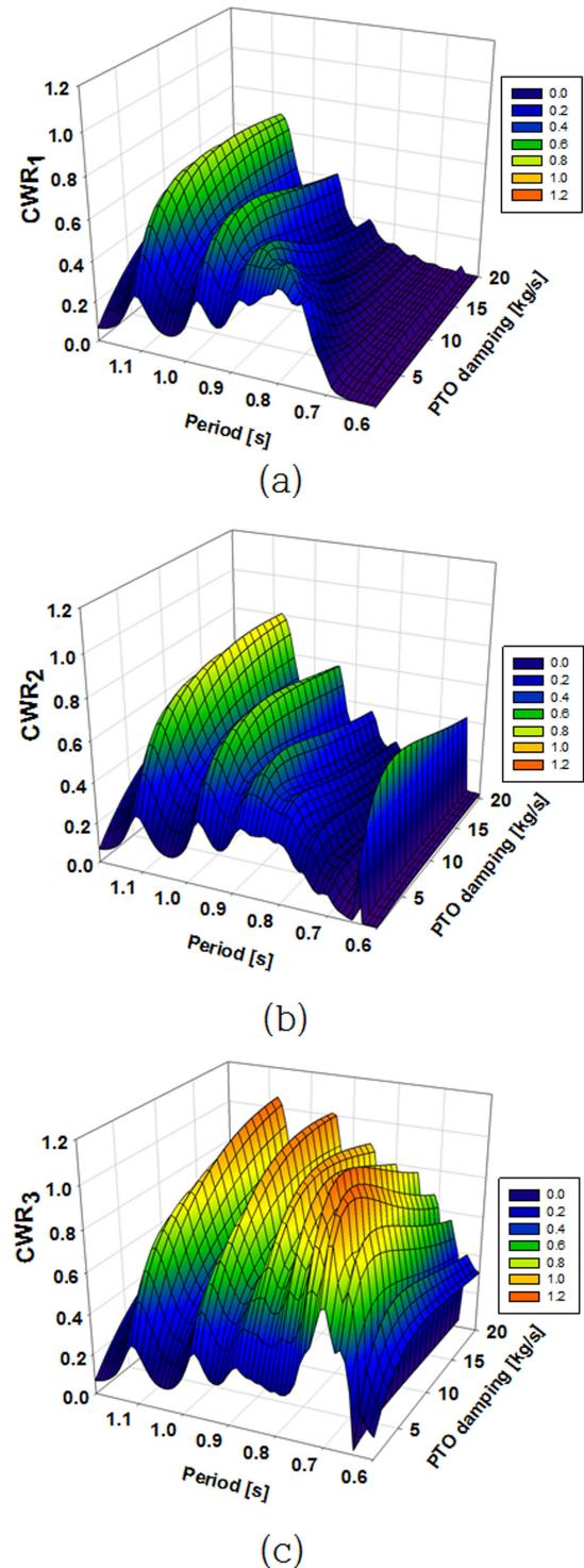
**Fig. 13.** Capture width ratio as a function of periods and PTO damping coefficients at three Cyl-1 cylinders arrayed in a water channel resonator.
