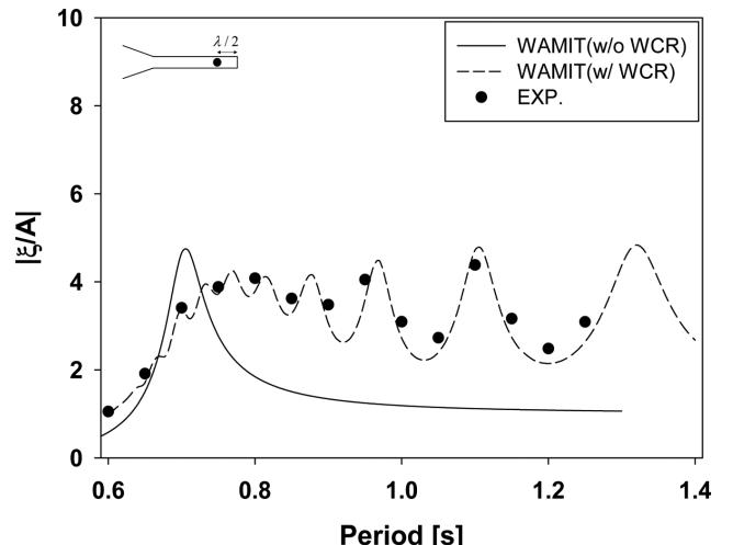
Fig. 8. Comparison of heave RAO between numerical solutions and experimental results with and without a water channel resonator for single Cyl-1 cylinder ( $b_{VIS} = 1.5376 \text{ kg/s}$ ).
