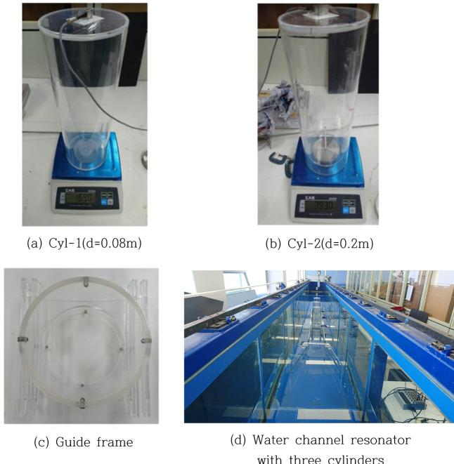
Fig. 2. Photographs of the experimental model.
